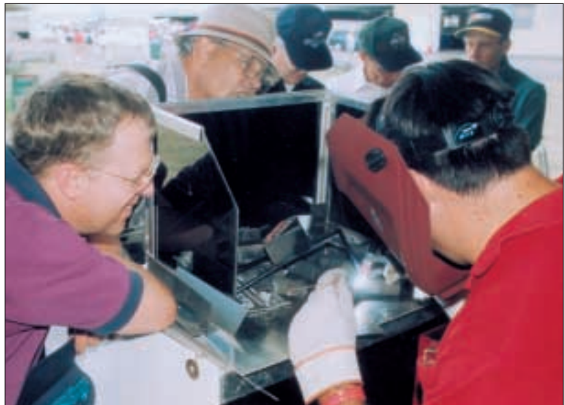
A demonstration of GTAW welding of 4130 tubing at the Experimental Aircraft Association Show in Oshkosh, WI.
